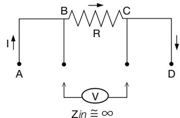
Four terminal (Kelvin) design: allows for precise and accurate measurements.
