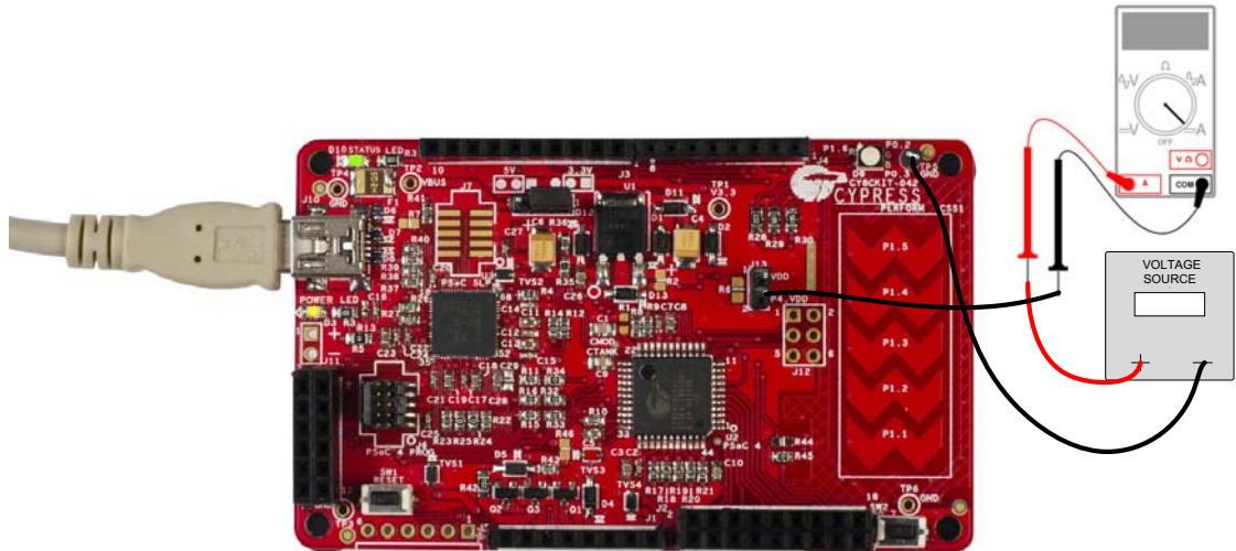
Figure 4-6. PSoC 4 Current Measurement when Powered Separately
