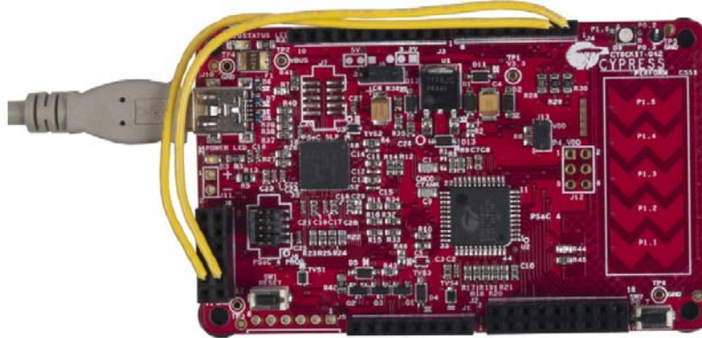
Figure 6-10. UART Connection Between PSoC 4 and PSoC 5LP
