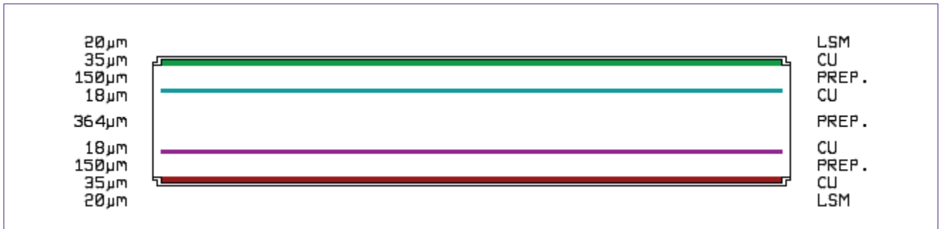
Fig 3. Layer stack of modified R_{th} -PCBs
