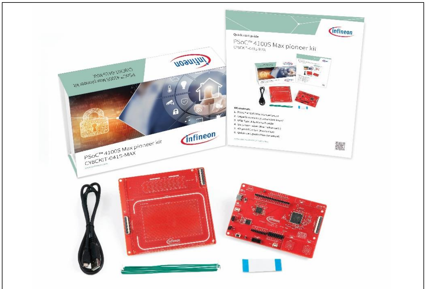
Figure 1 CY8CKIT-041S-MAX PSoC™ 4100S Max pioneer kit contents
