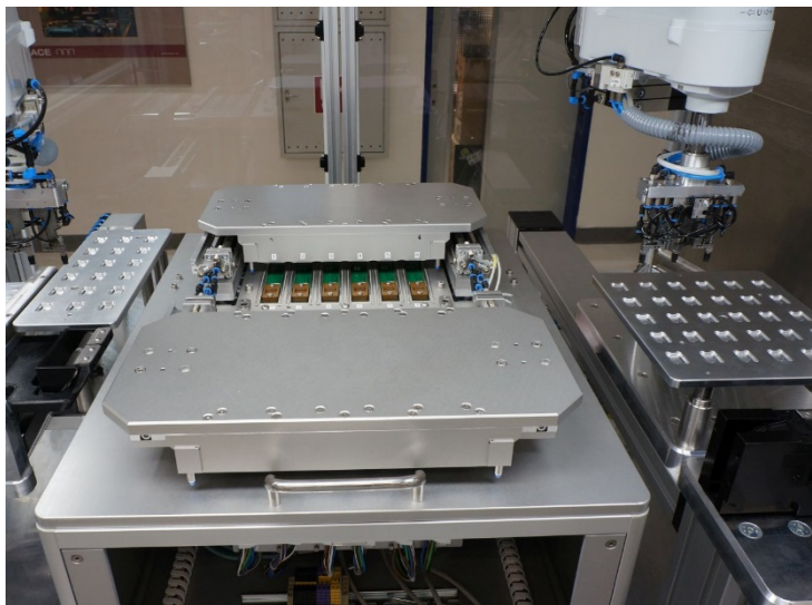
Figure 14: Automatic test equipment for module test
