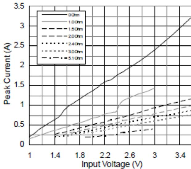
Fig. 2: Peak current vs. Input Voltage, for different values of external resistor
