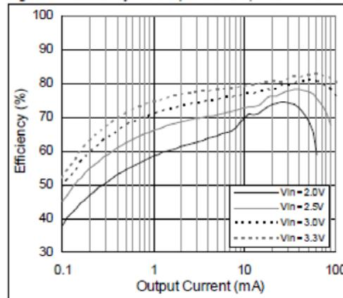
Fig. 3: Efficiency vs. Output Current for different Input Voltages of the AS1344
