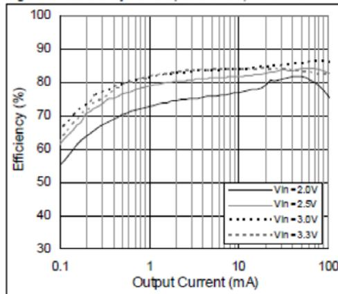
Figure 4. Efficiency vs. Output Current;  $V_{out} = 12V$
