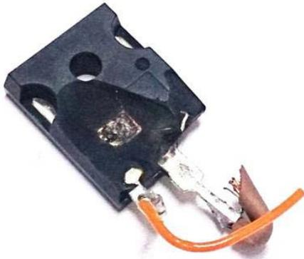
The ACPL-337J was electrically tested, and it passed the rated partial discharge test (1.88 kV<sub>RMS</sub>/s) and high voltage insulation test (6.2 kV<sub>RMS</sub>/s). Visual inspection was done externally and internally to determine the degree of damage to the insulation barrier.
