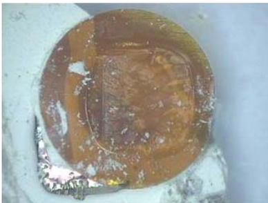
Optical inspection of the polyimide film showed no damage and the insulation remained intact.
