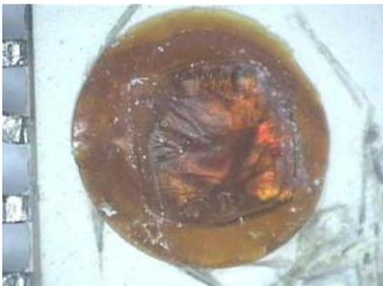
The ACPL-337J was electrically tested and passed the rated partial discharge test (1.88  $kV_{RMS}/s$ ) and high voltage insulation test (6.2  $kV_{RMS}/s$ ). There was no damage to the polyimide film and the insulation remained intact.
