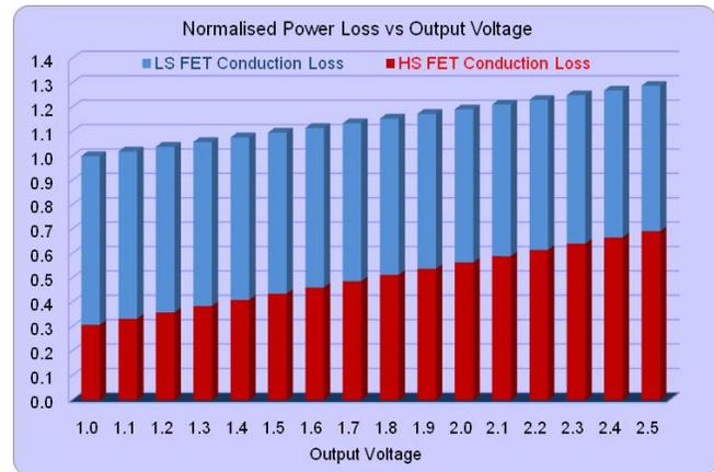
Fig. 8b. Normalised module loss vs output voltage
