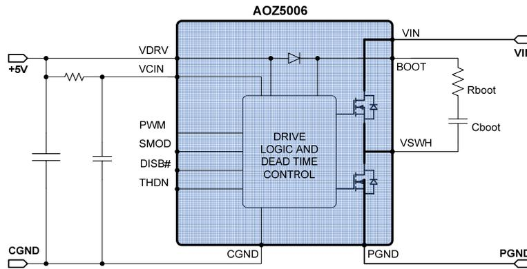
**Fig. 6. Connecting cboot and rboot for high side gate supply**
