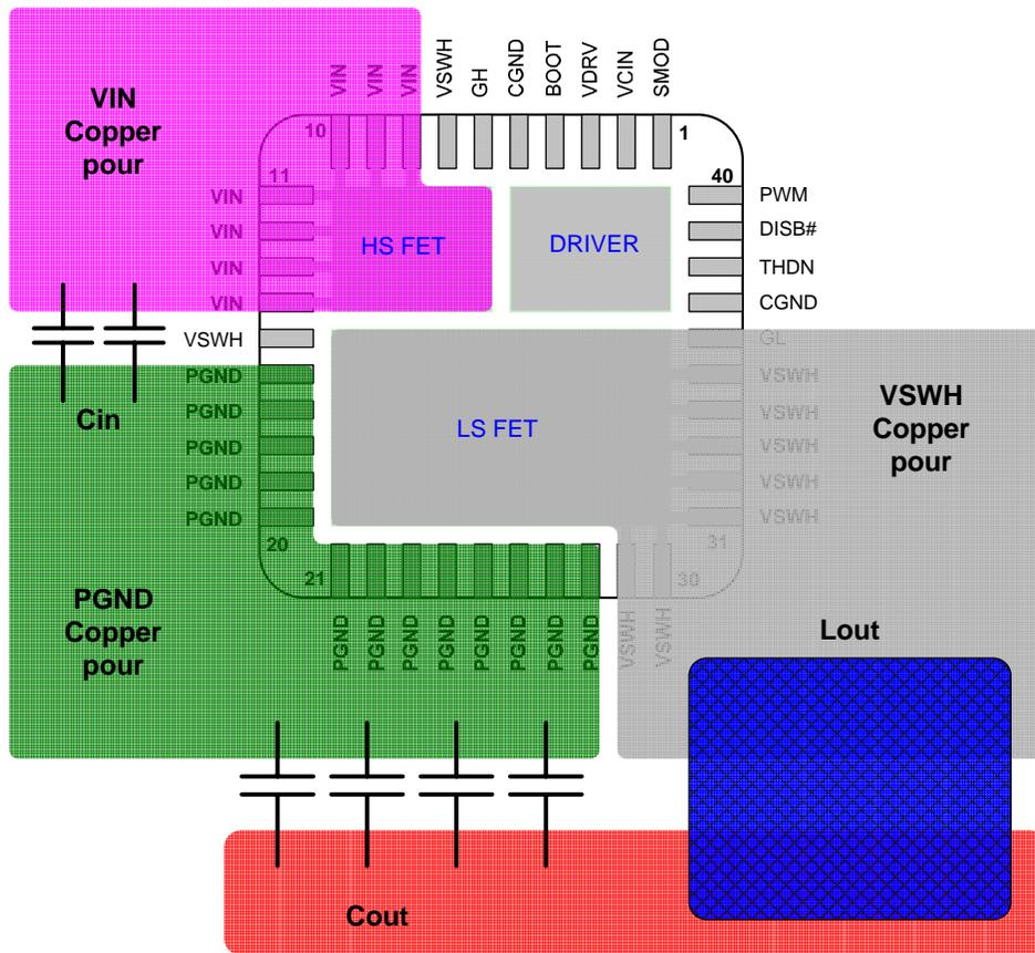
Fig. 9. PCB layout illustration for minimising current loops
