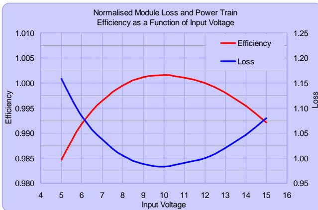
Fig. 8a. Normalised module loss vs input voltage
