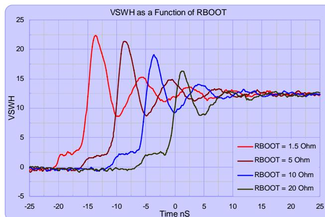
**Fig. 7. VSWH vs RBOOT resistor**
