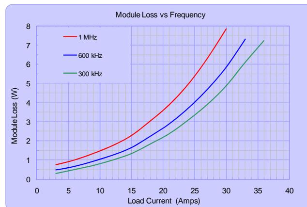
**Fig. 5. Module loss vs switching frequency**
