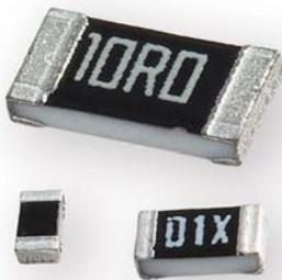
Yageo's thin film resistor RT series is a perfect solution for applications with high precision and high stability requirements. In thin film resistors, sputtering technology is used to form a nichrome (NiCr) resistive layer on the ceramic substrate. Compared to the printing process of thick film resistors, the metal resistive layer deposited by sputtering technology allows thin film
