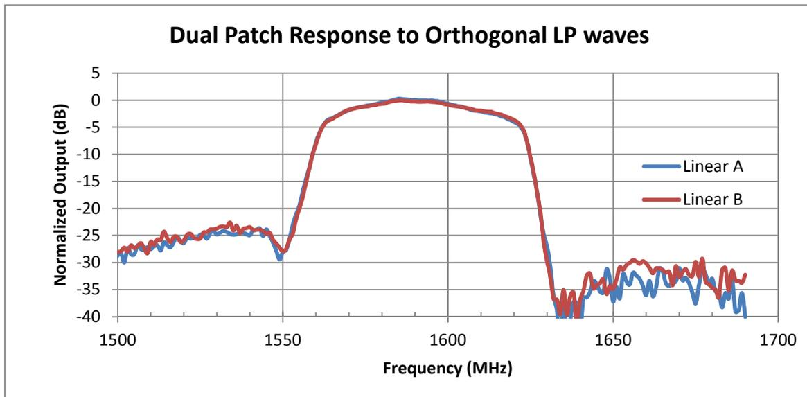
Fig 2(b), Normalized responses to orthogonal, linearly polarized waves
