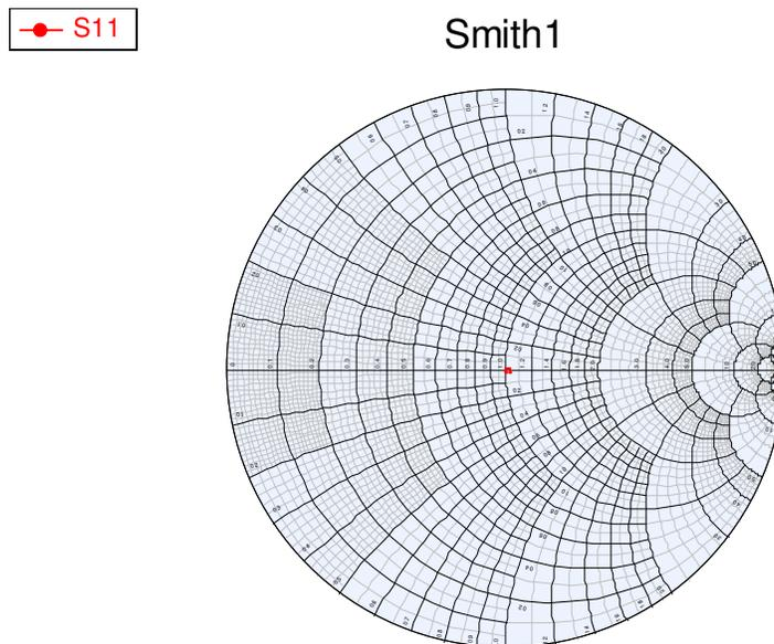
Fig 1 Simulated output impedance of dual feed patch with 90° hybrid summing network.
